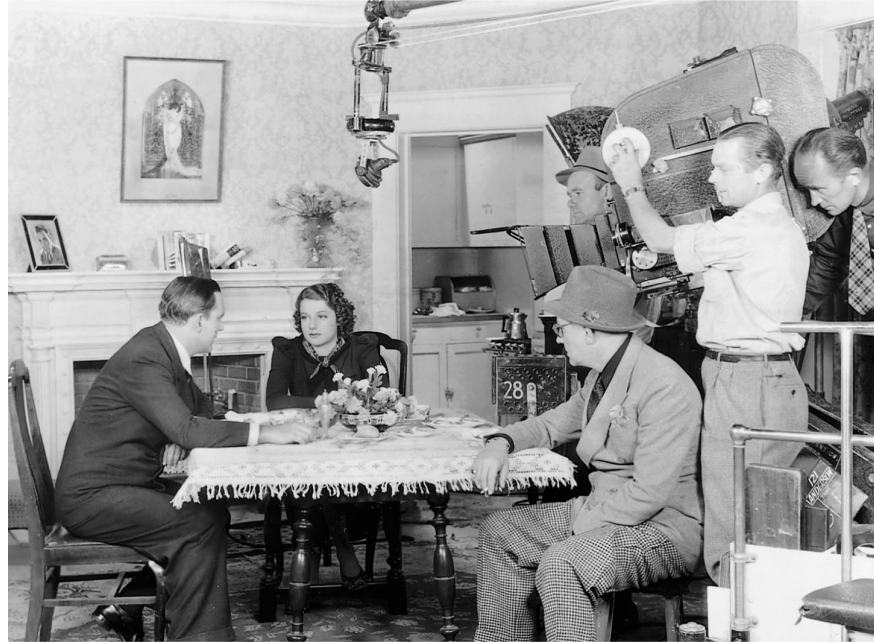
10.3 A lightweight boom aims a small microphone directly at the actors during production of Lloyd Bacon's San Quentin (1937). Note the padded metal blimp enclosing the camera.
