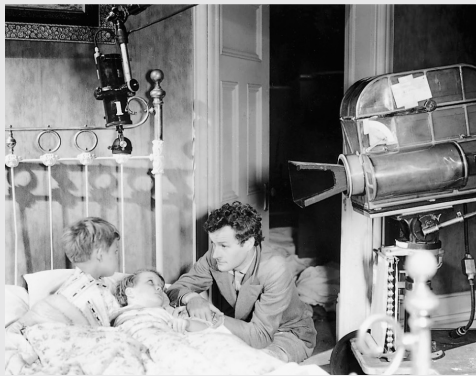
9.12 William Wellman directing The Star Witness (1931). The camera is muffled in a studio-built blimp, and the microphone hangs on a boom above the actors.
